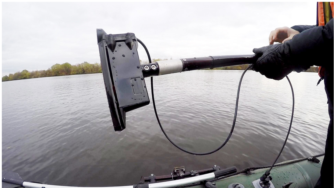
Figure J.1. Monoblock mount with KIT006
